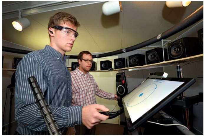
FIGURE 7. The experiment setup (a) includes 24 stimulus speakers evenly spaced in a ring with a diameter of eight feet. Larger speakers for background-noise output are shown in blue outside the ring, with a subwoofer shown on the right. The dashed line represents an acoustically transparent screen. The red-shaded speaker marks the direction directly in front of the listener, i.e., 0 degrees azimuth. The photograph in (b) shows the actual system, including the touch screen, with the acoustically transparent cloth removed to expose the loudspeakers.
